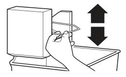
**NOTE:** Turn off the ice maker before removing the ice storage bin to serve ice or to clean the bin. This will keep the ice cubes from dropping out of the ice maker and into the freezer compartment. After replacing the ice storage bin, turn on the ice maker.
