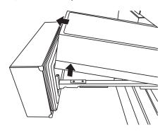
2. Left-hand drawer only: Remove the wiring connection cover. Press in on the side of the cover to release the tab from the slot, and then pull the cover away from the bracket.
