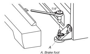
Make sure the refrigerator is steady. If the refrigerator seems unsteady or rolls forward when a door or drawer is pulled open, adjust the brake feet.
