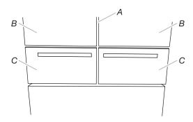
Aligning the drawer fronts is a two-step process. The first step is to adjust the drawer fronts up and down. The second step shifts the drawer fronts from side to side. Visually inspect the refrigerator for alignment and adjust the drawer fronts as needed.
