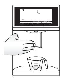
4. When 1 cup of water has been correctly dispensed into the measuring cup, press the Measured Fill button under the word "Confirm" to confirm the calibration.
